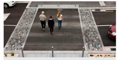
Example of a raised pedestrian crossing with 'rumble' pavement edges and kerb outstands. Taradale, New Zealand
